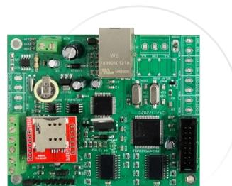
CPU PER LA GESTIONE CON CONNESSIONE LAN ETHERNET
